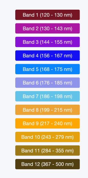
LUMA acquires data in discrete wavelength band from 120nm to 500nm. This broad range includes the Vacuum Ultraviolet (VUV)) Region of the electromagnetic spectrum. This region is unique because all compounds absorb except for typical GC carrier gases Hydrogen, Helium, and Argon.
