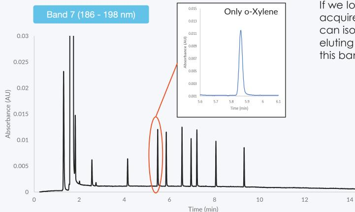
If we look at the chromatogram acquired in Band 7 (186 – 198 nm) we can isolate o-Xylene since the coeluting compound does not absorb in this band.
